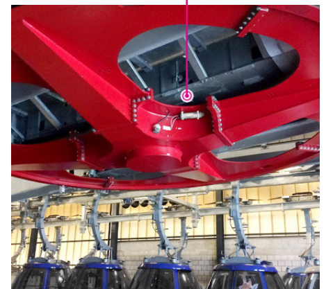
In the valley station, the deflection roller of a chairlift is lubricated with two simalube 250 ml lubricators.
