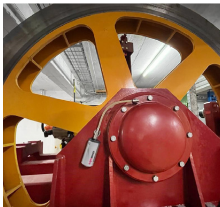
Pulleys can be lubricated automatically, easily and reliably with a 125 ml simalube via a hose.
