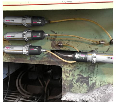
Thanks to the simalube IMPULSE pressure booster, the lubrication points at the winder (bearings, guide bushes and interlocks) can be installed remotely and supplied with lubricant via a hose installation.
