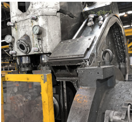
Several simalube lubricators and IMPULSE lubricate the columns (left) and the drive unit (right) of the nibbling machine.
