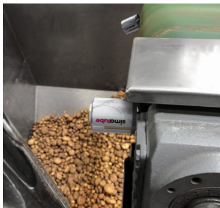
Two 60 ml simalube units lubricate the bearings of the deflector roller of a conveyor belt in potato processing.
