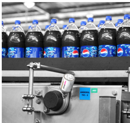
Lubrication of a flange bearing on a filling machine for soft drinks.
