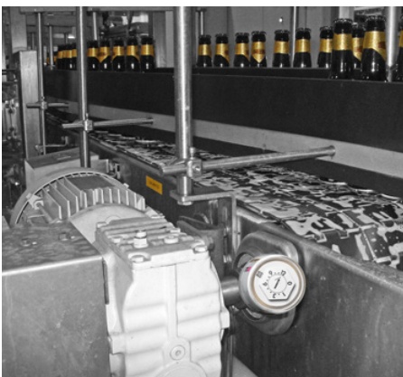
Lubrication of a transport belt with a simalube lubricator.
