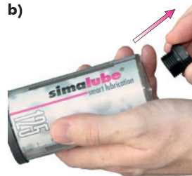
b) Remove gas generator with a socket wrench (SW21 mm)
