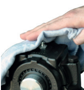
Clean lubrication point
