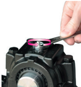
Remove connector nipple
